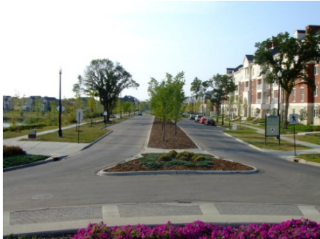
Example of walkway and street designed for pedestrian safety and enhanced aesthetics. Edmonton (source: Cory Labrecque)
